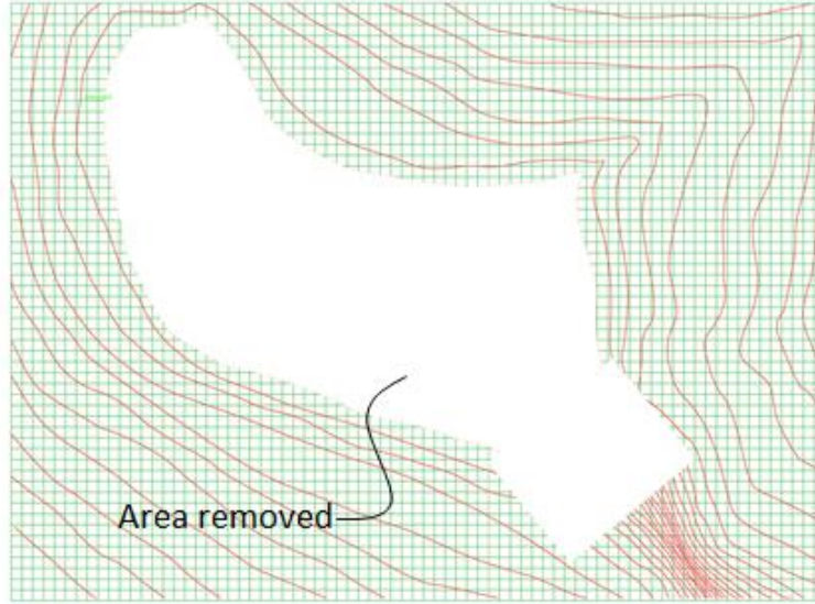
Both the area representing the water surface and the dam are removed from the DEM.
