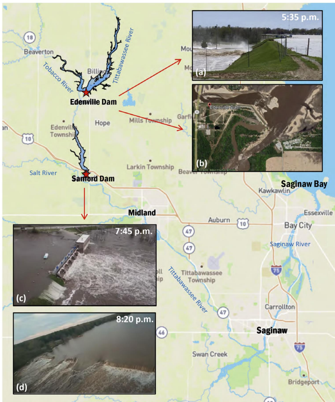
Figure 2 Edenville and Sanford Dam Locations and Images of (a) Edenville Dam Breach (Coleman, 2020), (b) Edenville Dam After the Failure (Google Earth, 2022), (c) the Fuse Plug Spillway of Sanford Dam Being Overtopped (CFI Media (Checkeder Flag Interactive Media), 2020), and (d) the Entire Embankment of Sanford Dam Being Overtopped (Michigan Drone Services)
