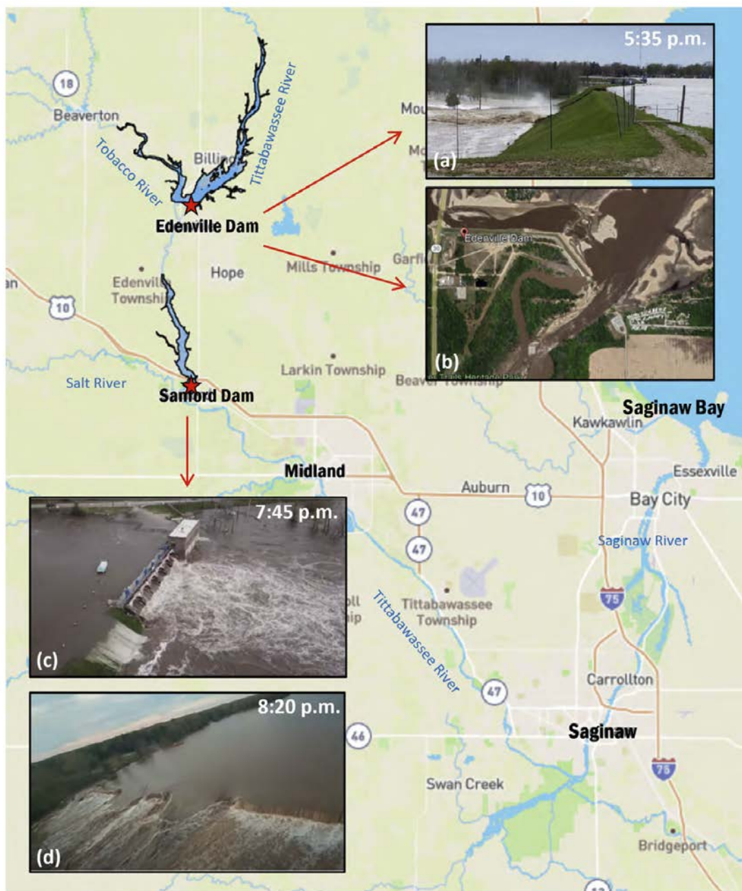
Figure 2 Edenville and Sanford Dam Locations and Images of (a) Edenville Dam Breach (Coleman, 2020), (b) Edenville Dam After the Failure (Google Earth, 2022), (c) the Fuse Plug Spillway of Sanford Dam Being Overtopped (CFI Media (Checked Flag Interactive Media), 2020), and (d) the Entire Embankment of Sanford Dam Being Overtopped (Michigan Drone Services)
